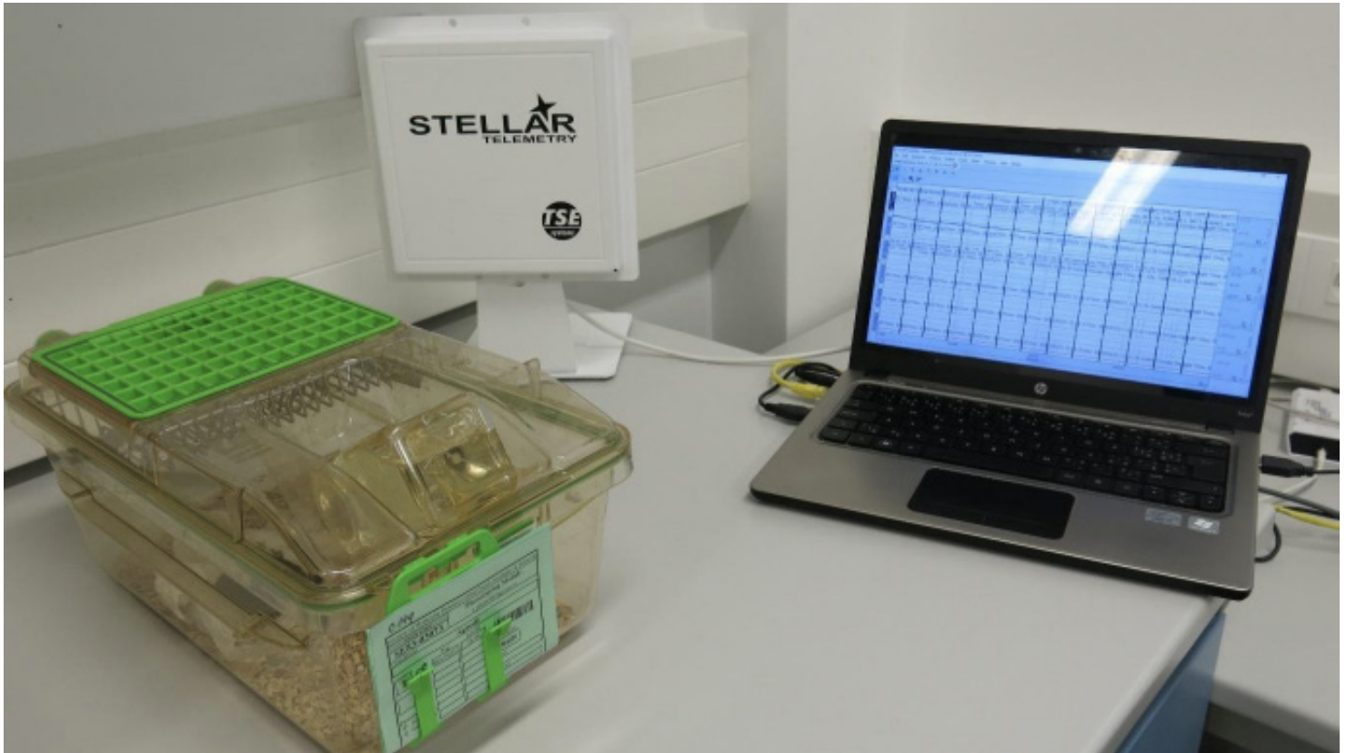
Telemetry System measuring 2 different temperatures in a non-restrained mouse
